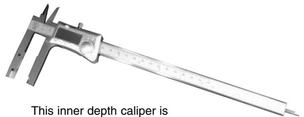
This inner depth caliper is with five modes of measurement (OD, ID, General Depth, Groove Width, and Groove Depth). It has a digital display capable of displaying mm, inches, and fractions and can take measurements of up to 8" (205 mm). The four groove depth pins located on the back of the calipers measure 10mm, 20mm, 3/8", and 3/4".
